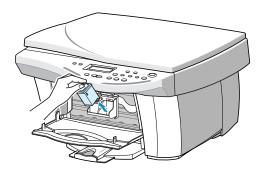
**4** Use a CLEAN, DRY CLOTH to clean the print cartridge contacts inside the printer.
